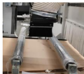
Pressing roller for helping hold small panels
