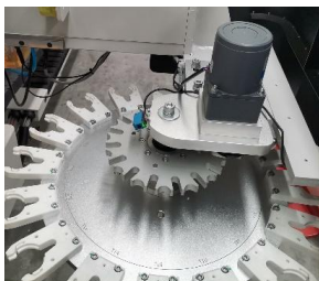
Carousel 16-slot, stepper motor, fast and efficient in tool changing.
