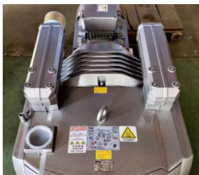
2 x 4kw pumps with strong suction capacity, holding the panels firmly during processing, no movement, no waste of panels
