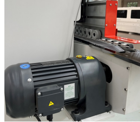
Heavy Duty motor used for the conveyor chain
